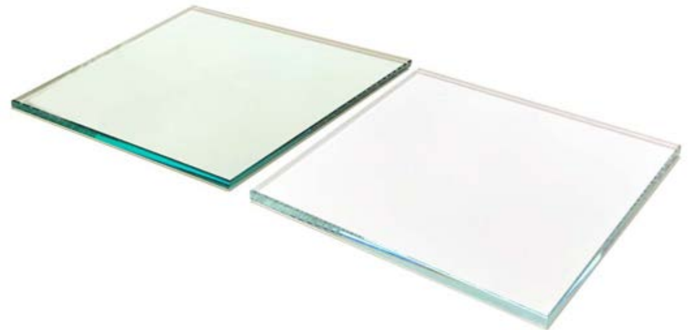
Figure 3.17. The difference between clear glass (left) and low iron glass (right).
