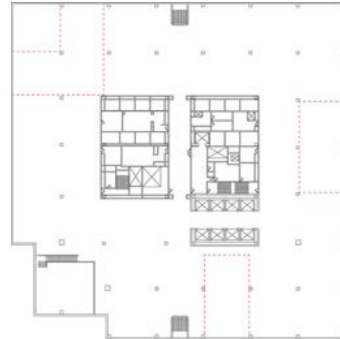
Figure 3.14. Example of possible floor cut locations.
